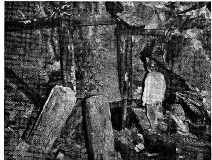
Figure 8.—Stope on North orebody, showing wall of diagonal fault in upper right cutting ore in middle background. Picture taken in 1941.
