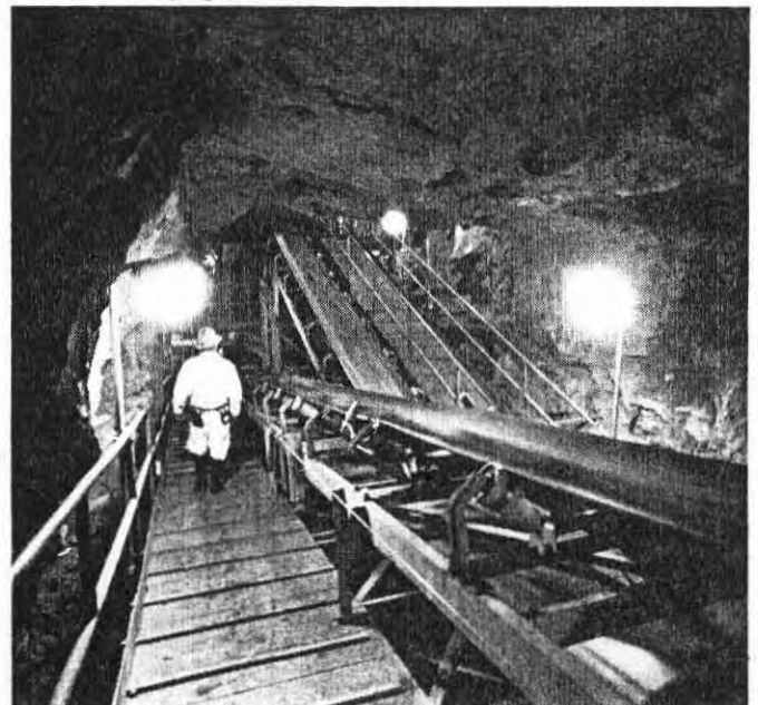
Goldstream. Conveyors are part of underground crushing and screening system
