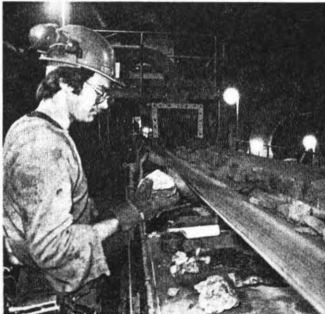
Goldstream. Conveyor from screens returns oversize to crusher
