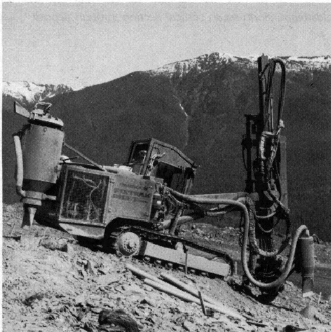
Goldstream. Tamrock Fixtrack DHA Turbo drill used for blasthole drilling in the open pit
