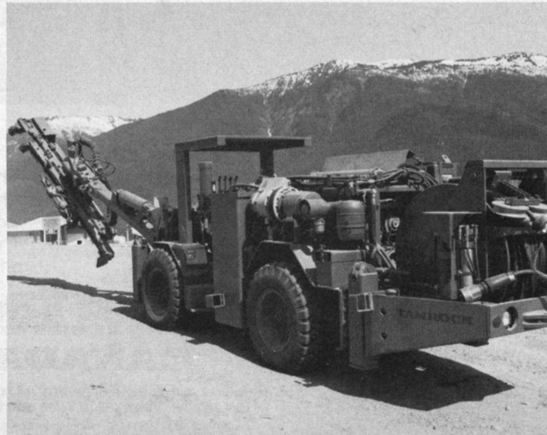
Goldstream. Two Tamrock Minimatic H107L electro-hydraulic drill jumbos will be used for underground mining development
