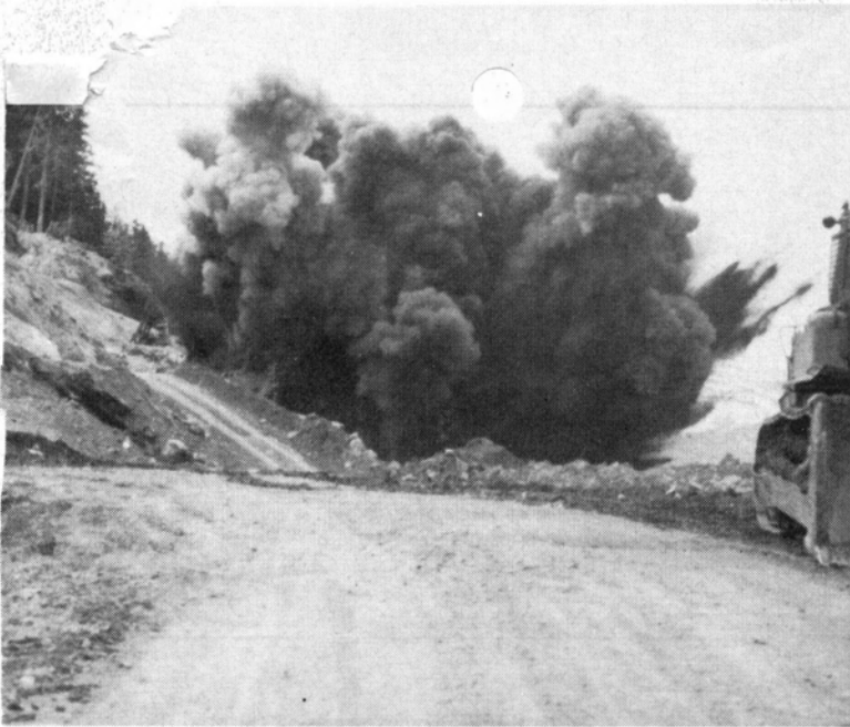
Goldstream. Open pit blast when the ore is broken into small pieces of more than eight tons (four tons for additional recovery).
