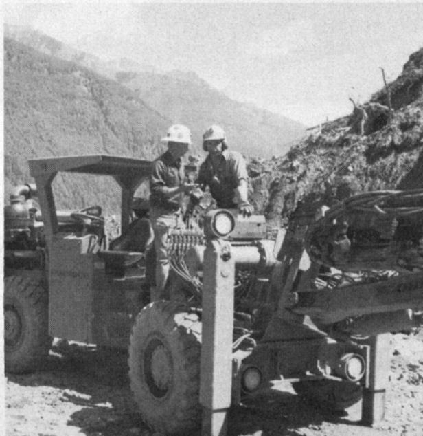
Goldstream. Tamrock Minimatic DH107L drilled the first round
