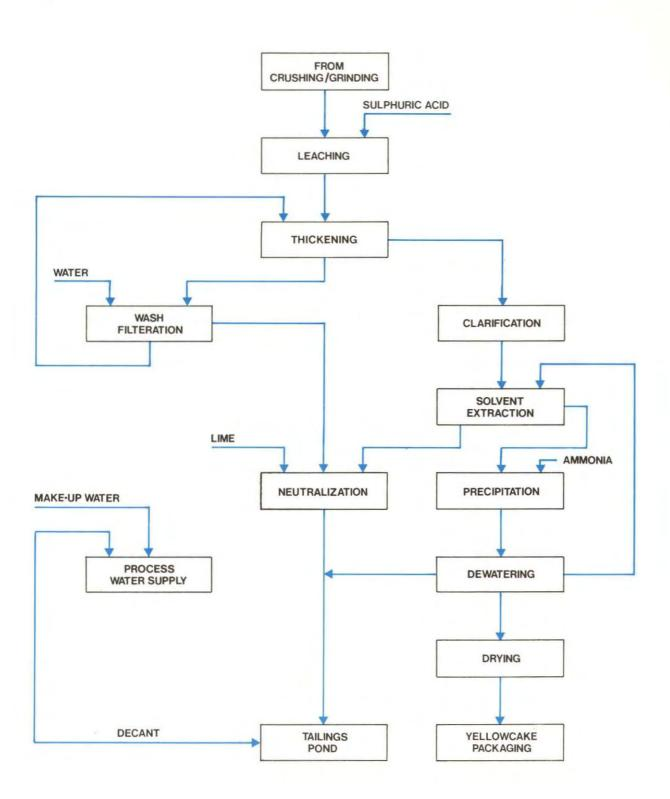
PROPOSED HYDROMETALLURGICAL CIRCUIT
