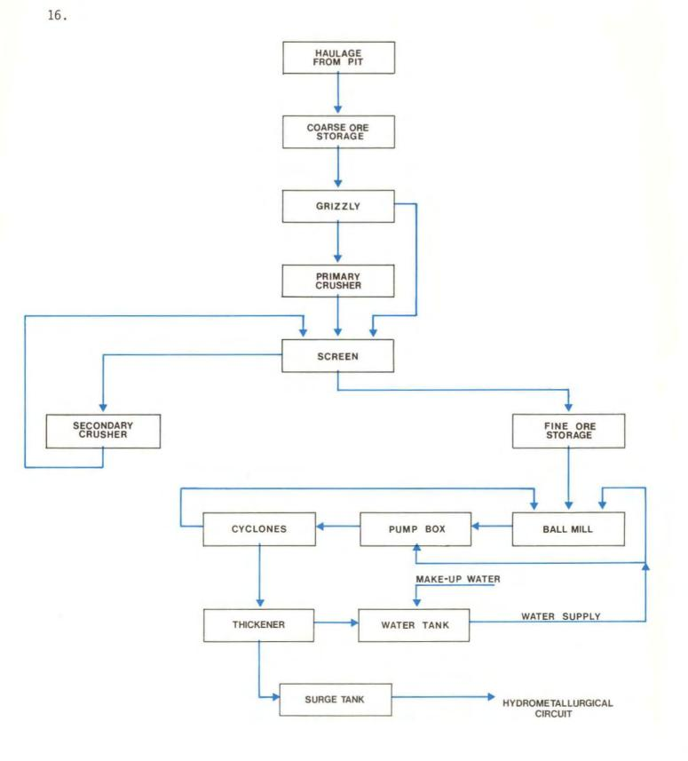
PROPOSED CRUSHING / GRINDING CIRCUIT
