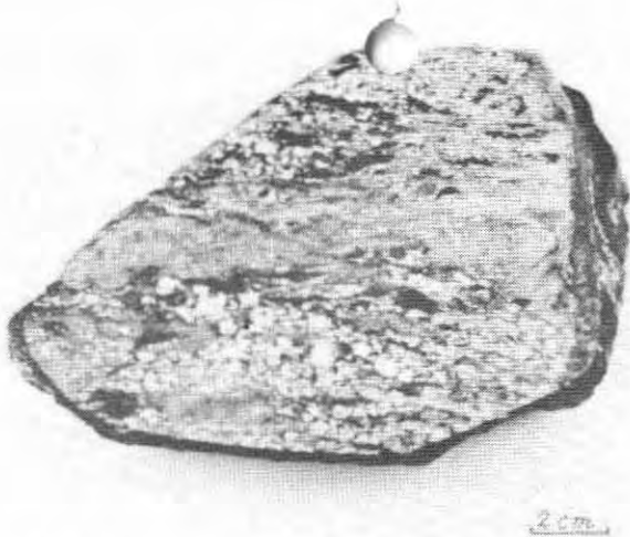
PLATE 7A — Ore from the Rexspar A zone, showing sheared pyrite and fluorite (dark grey).
