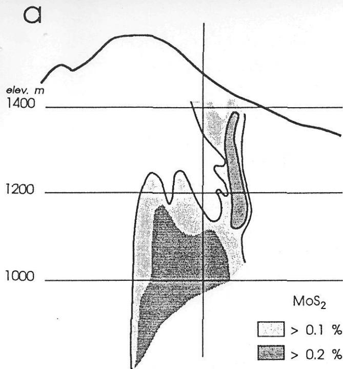
FIGURE 7a. Cross-section along the adit of the Trout Lake deposit showing results from drill core pulp analyses (containing wallrock and veins) — contours of MoS<sub>2</sub> grade. Modified after Boyle and Leitch (1983).
