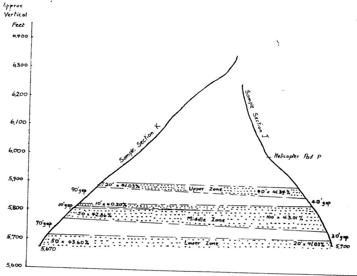
Schematic Section in Mountain Slope at J-K Location
