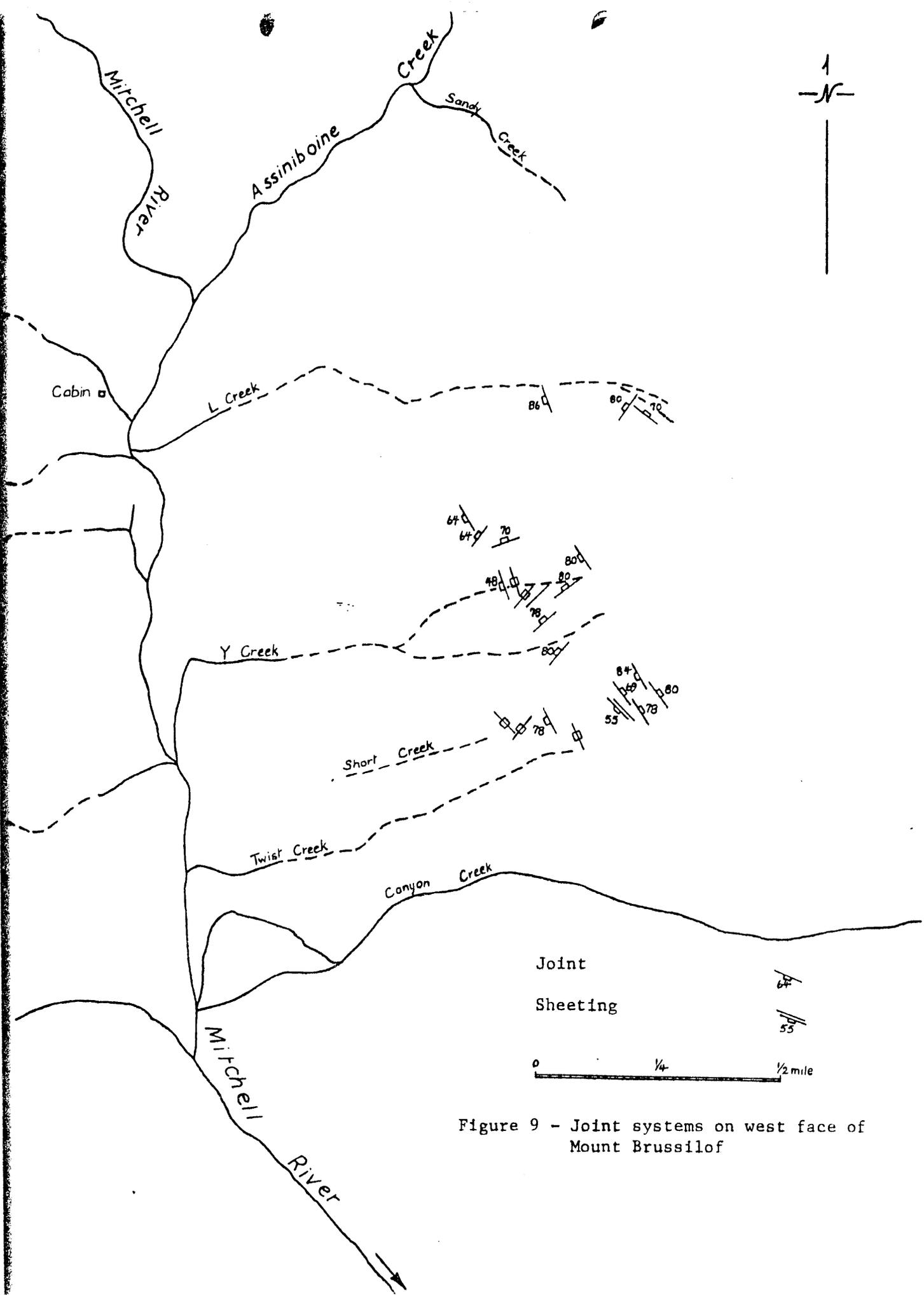
Figure 9 - Joint systems on west face of Mount Brussilof
