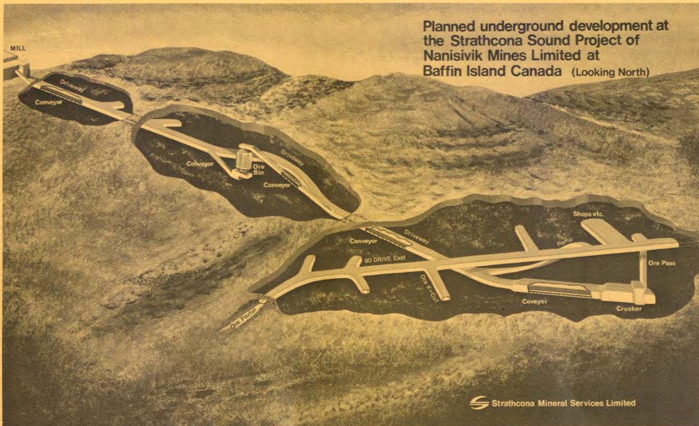
Cut-away view of room and pillar mining at NANISIVIK MINES LIMITED Strathcona Sound N.W.T.
