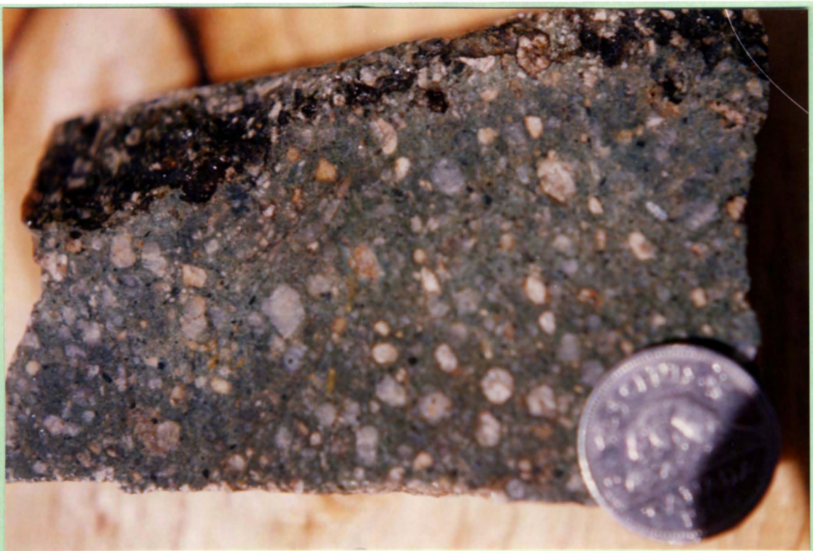
14. GREEN, COARSE GRAINED PORPHYRITIC SYENITE WITH AEGIRINE AND AEGIRINE - AUGITE HOWELL CREEK
