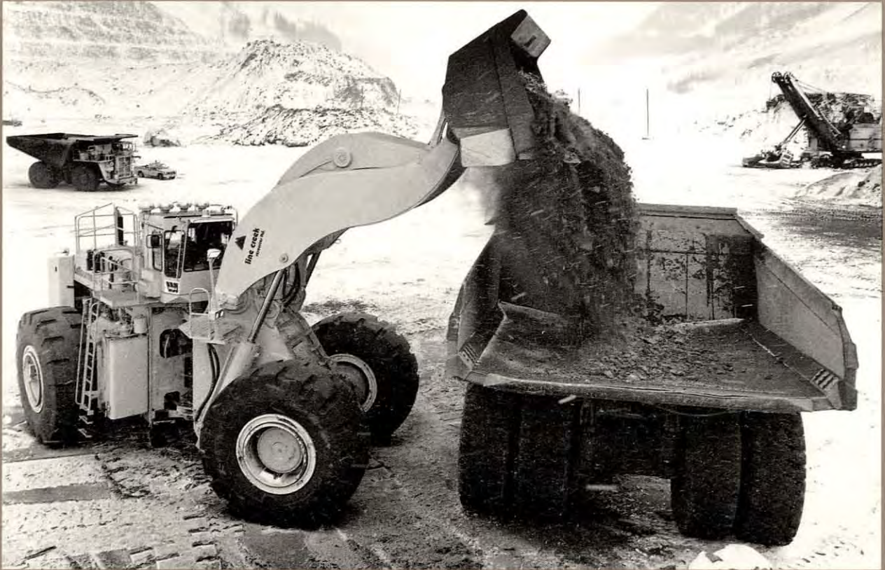
New LeTourneau L1400 with 22m 3 bucket is among the largest loaders operating in Western Canada.
