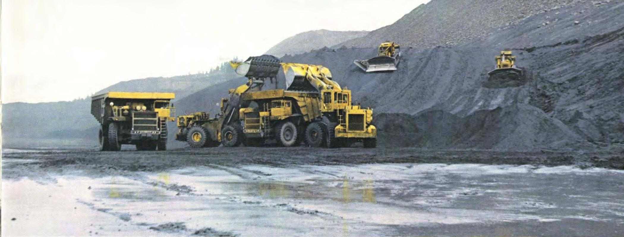
*Coal is pushed off the seam with dozers, loaded into 100-ton trucks and hauled to the central breaker station.*
