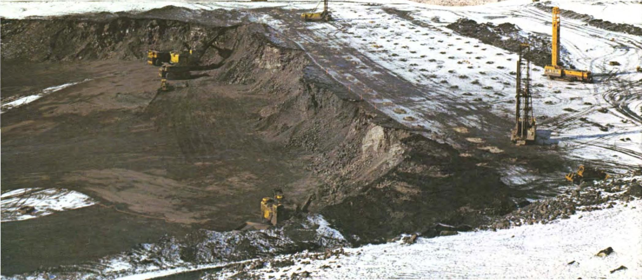
**DRILLING AND BLASTING** is the first stage in removing the rock overburden. Large rotary drills produce blastholes 12¼ inches in diameter and 50 feet deep. Explosives are delivered to the holes from an on-site bulk loading and storage facility.
