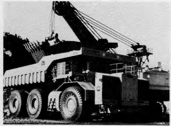
The world's largest truck, the 350-ton Terex 33-19, is on trial at the surface coal mining operations of Kaiser Resources at Sparwood, B.C., to determine its performance as an overburden hauler.
