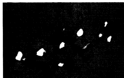
Cluster of free gold grains (10-30 microns) in Bedrock Sample from Gold Mountain Discovery.
