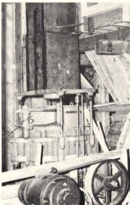
Salmo: Cone crusher in tungsten mill
