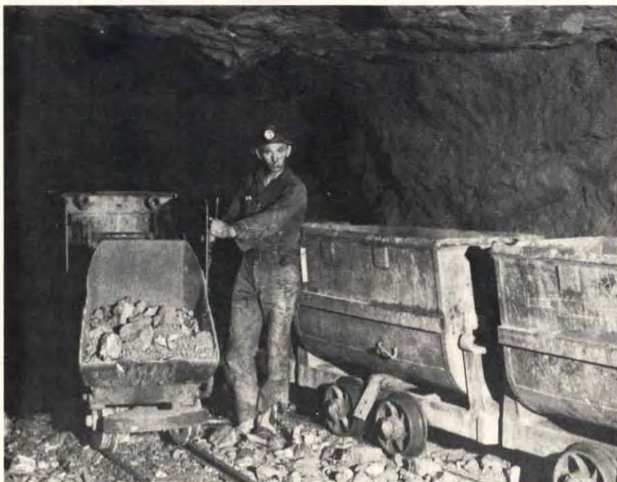
Salmo: Mucking machine operating in a drift slash
