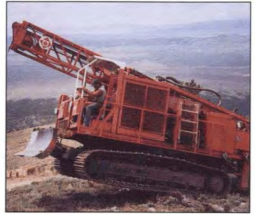
At Mount Hamilton, track mounted drill rigs have been used for off-road drilling with minimal environmental disturbance.
