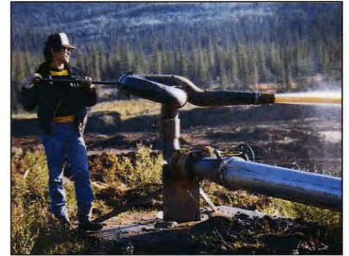
Queenstake uses water monitors such as this hydraulic set-up at Maisy May Creek to inexpensively remove thawed overburden from pay gravels.
