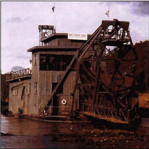
A Queenstake 350 ton bucketline dredge in operation at Clear Creek, Yukon.
