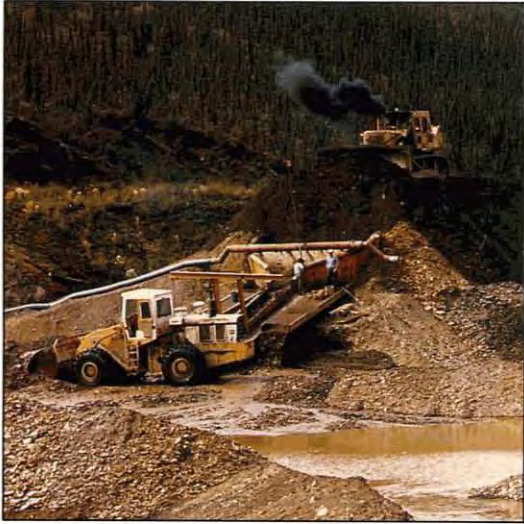
Yukon placer operation: Bulldozers push pay gravels to the sluice box where a 3,000 gallon per minute water flow washes the gravel over a series of riffles, trapping the heavy gold particles. A loader removes and stacks the tailings.
