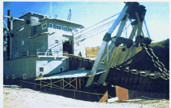
Dredge #4 in Bonanza Creek, Klondike Mining District: a relic of the rich placer mining that continued by dredging to the mid 1960's
